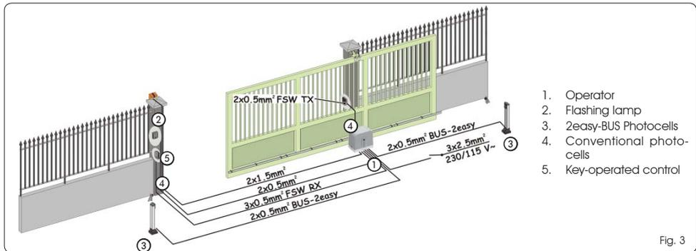
The dimensions and electrical preparations (standard system) are the same for operator C720 and for operator C721
