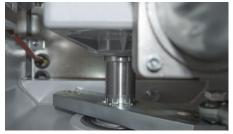
Drive of the boom shaft directly by the geared motor for easy adjustment.
